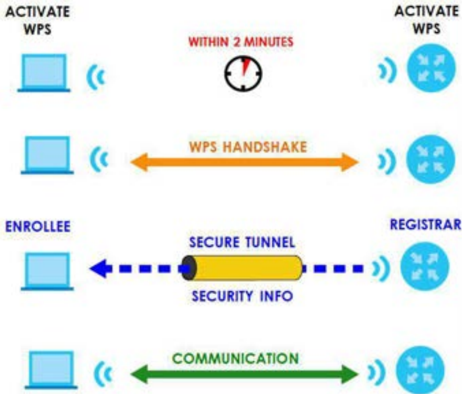
Figure 59 How WPS Works
